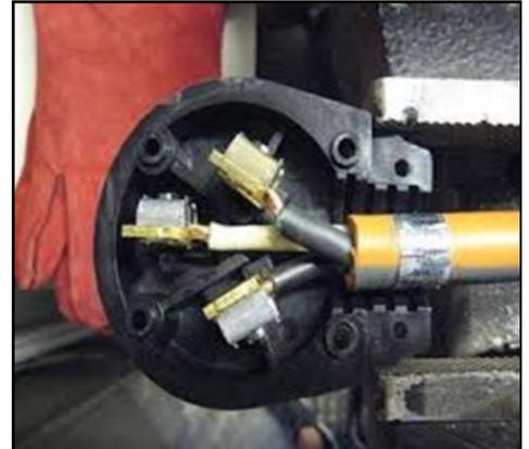
Any cord with exposed wires should be immediately destroyed and replaced with a new cord. Touching even a single exposed strand can result in an electric shock or burn. Always insert plugs fully so that no part of the prongs are exposed when the extension cord is in use. Do not nail or staple cords to walls or baseboards or hang them in such a fashion that will not damage the outer jacket or insulation.
