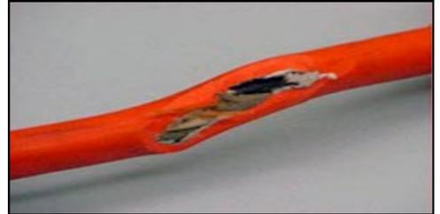
Verify that the right type and length of cord is being used for the application, environment, and power demands. Check the outer jacket and cord ends. If they feel warm or hot, immediately discontinue cord use. This may indicate overloading or internal damage. Internal damage may also be present if the outer jacket was pinched or crushed, the ends are damaged or tape has been placed over the outer covering. See **Appendix 1** for a *Model Extension Cord Inspection Checklist*.
